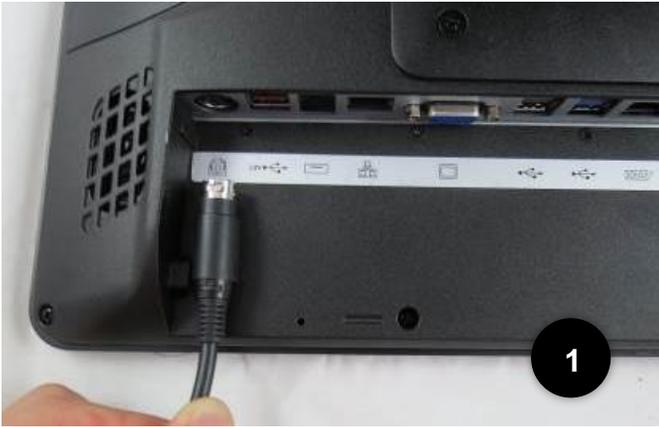
1. Connect cable to DC-in 12V
